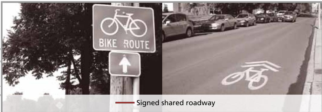
Standard road with a combination of traffic calming, signage and “sharrows” (shown at right), or a high-volume road with 14-foot or wider outside lanes.
